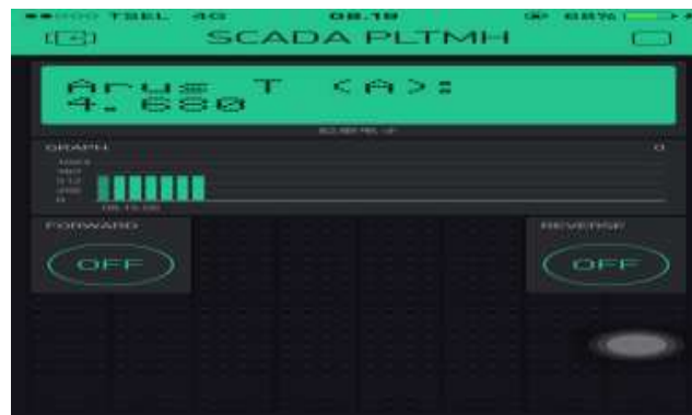
Figure 3. Monitoring Measurements on Phase T using ACS712 30A current sensor with smartphone.
