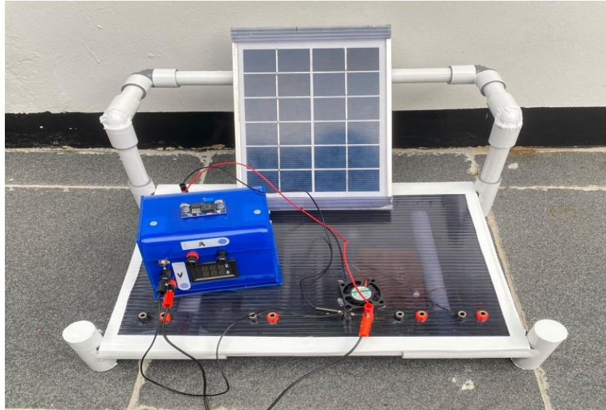
Figure 2 <Renewable Energy Instructional Aid Product in the Form of a Solar Power Plant (PLTS)>
