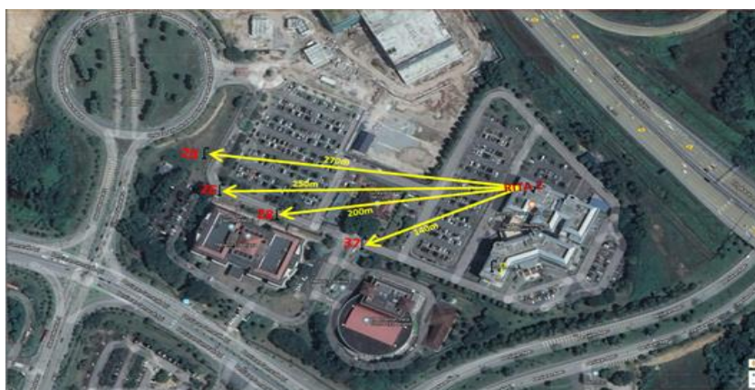
Figure 4 <LoRa-based Distance between the Four controllers and the Gateway (RITA)>
