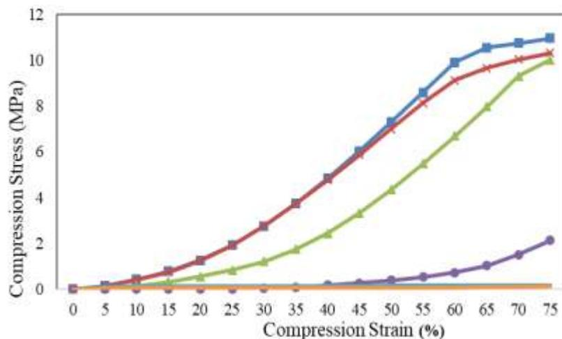
**Figure 2.** Compression Stress Versus Compression Strain of MR Fluid Samples
