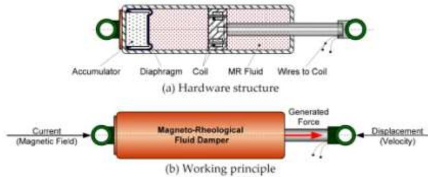
**Figure 1.** Damping Mechanism on a Car (a) Hardware Structure (b) Working Principle (Truong & Ahn, 2012)
