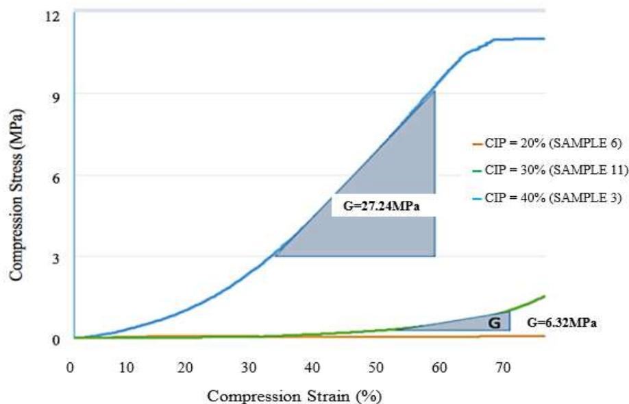
**Figure 3 Compression Modulus of MR Fluid**
