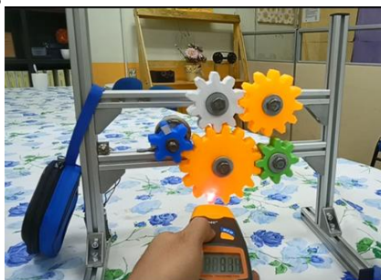
Figure 8 <Testing and Measure RPM by Using Tachometer>
